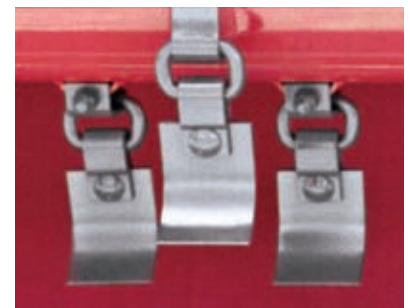
32 high-vacuum knives provide cutting and blowing action, eliminating separate conveyors and blowers.
