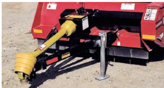
A constant-velocity P.T.O. shaft protects the driveline during turns, reducing wear on drive components.
