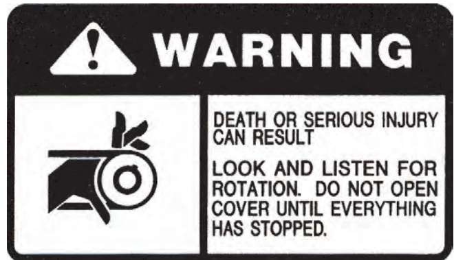
FIGURE 23 71505169 Warning: Look and Listen...
