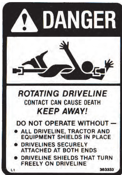
FIGURE 27 520-03138 Danger: Rotating Drive...
