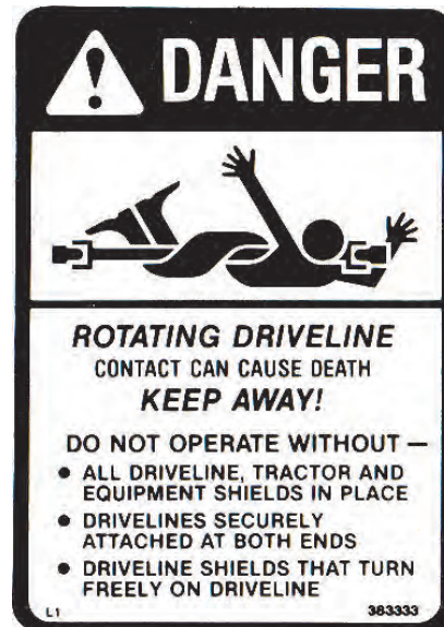
FIGURE 22 520-03138 Danger: Rotating Drive...
