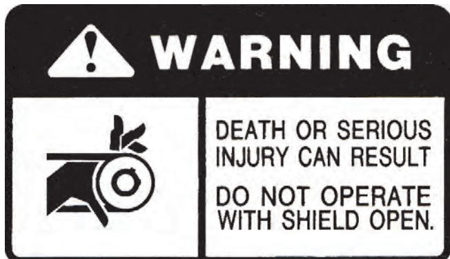
FIGURE 28 71505170 WARNING: DO NOT OPERATE...
