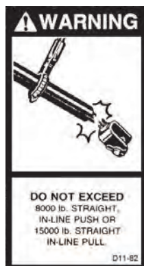
FIGURE 29 WARNING: DO NOT EXCEED...
