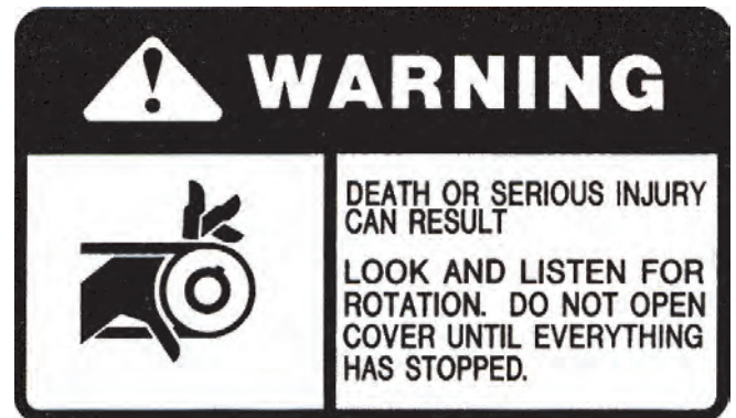
FIGURE 12 71505169 Warning: Look and Listen...
