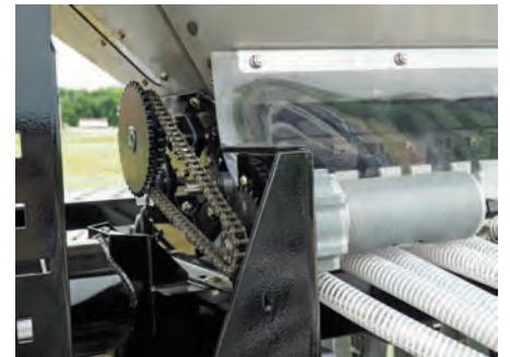
Metering drive choices include variable rate hydraulic or variable rate 12-volt electric (shown).
