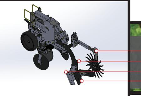
Rotary Hoe Shield Liquid Fertilizer Y-Tube Point and Reversible Share Ridgers
