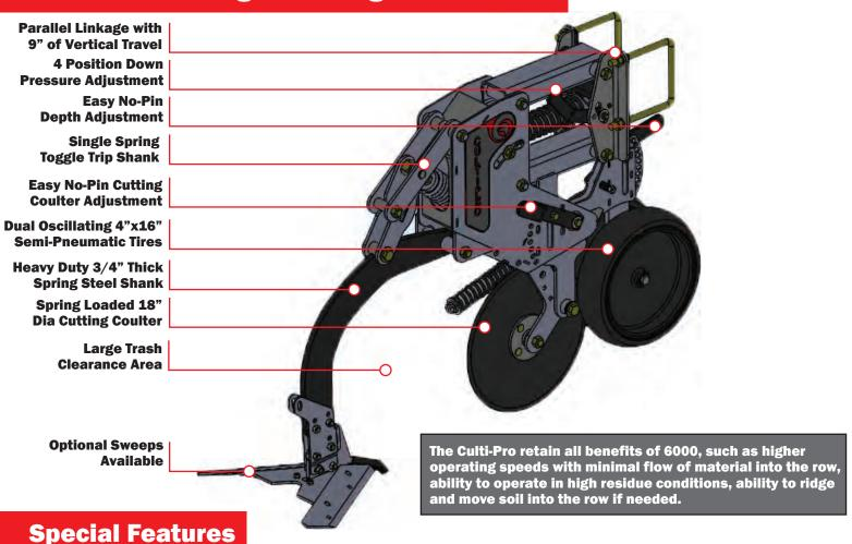
11.5 inches in length added to improve trash flow between cutaway discs and shares. Narrower row unit structure with <sup>3</sup>/<sub>4</sub>" spring steel flat shank accommodates narrower 20" row spacing. Ability to adjust pitch of the share assembly. Quick, easy, no tool, hand adjustments.
