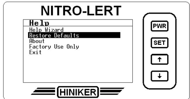
The Restore Defaults option is used to reset the Nitro-Lert to its factory default settings.
