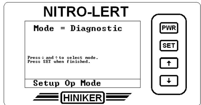
Use the ↑ and ↓ keys to toggle between the two modes. Press SET when done. Diagnostic is default.
