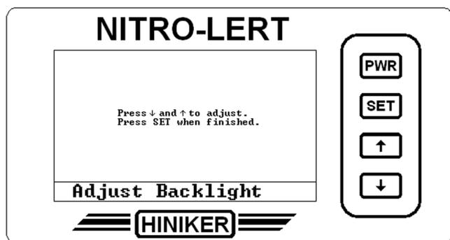
Press the ↑ key to increase the brightness of the display backlight or the ↓ key to decrease the brightness of the display backlight. Press the SET key to lock in the setting and exit the screen.
