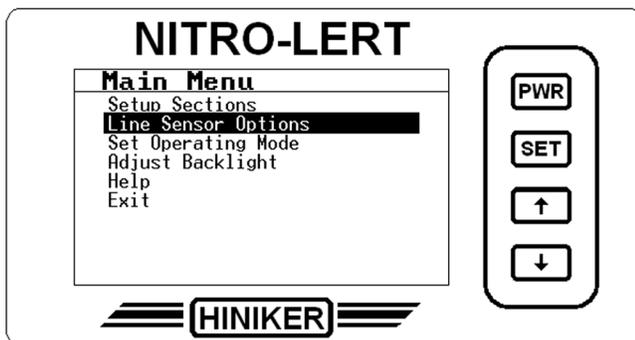
This option allows you greater flexibility in controlling individual lines. Here you have the ability to set a line as in normal operation (Active), monitored only (MON) or ignored (OFF).
